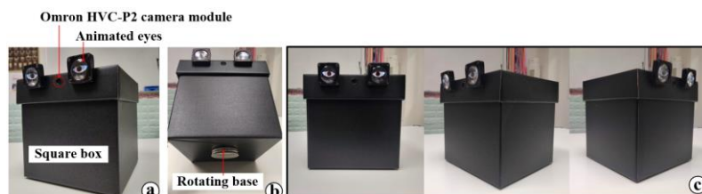
Figure 2. (a) Square box mounted with animated eyes and Omron HVC-P2 camera module, (b) rotating base attached at the bottom of the box, and (c) square box turning towards the user.
