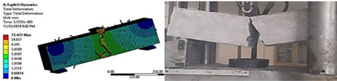
Figure 12. Comparative analysis of concrete beam (FRC 5)
