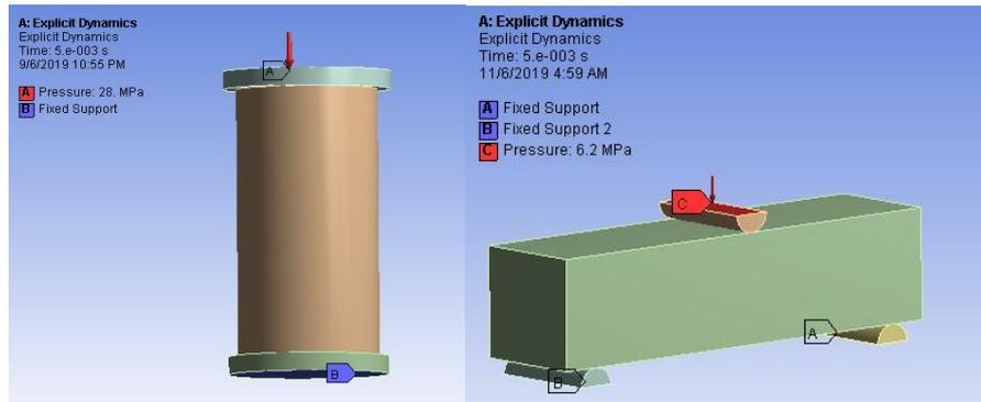
**Figure 1.** Boundary condition for compressive and flexural strength evaluation
