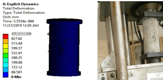
**Figure 5.** Comparative analysis of concrete cylinder (FRC 6)
