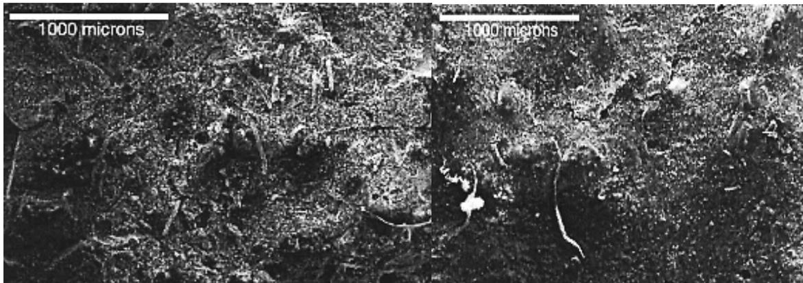
**Figure 15.** Scanning Electron Microscope Micrographs of fracture surface
