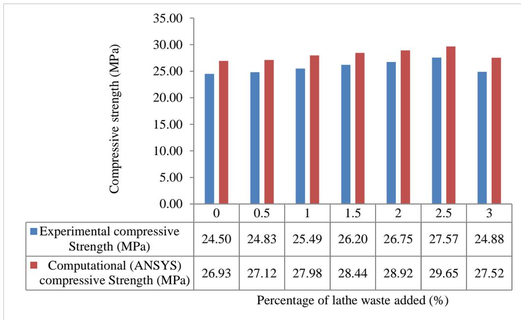
**Figure 6.** Destructive compressive strength vs Computation Analysis
