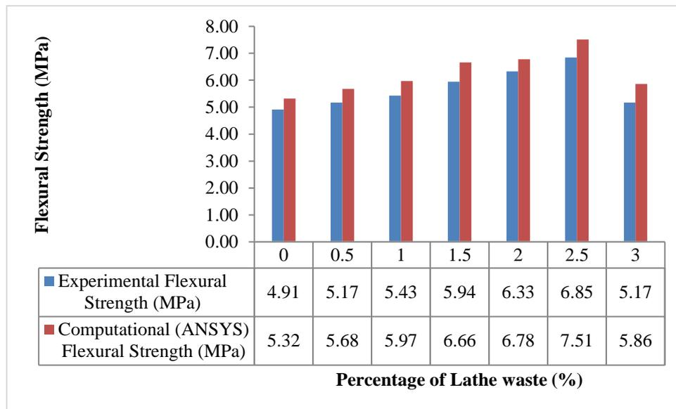
Figure 14. Destructive Flexure strength vs Computation Analysis
