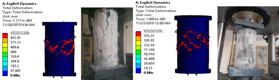
**Figure 4.** Comparative analysis of concrete cylinder (FRC 4 & FRC 5)
