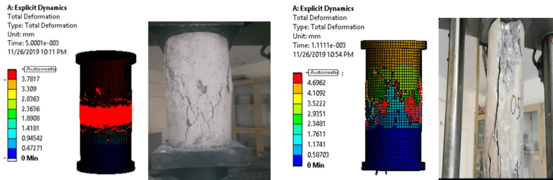
Figure 2. Comparative analysis of concrete cylinder ( $M_0$  & FRC1)
