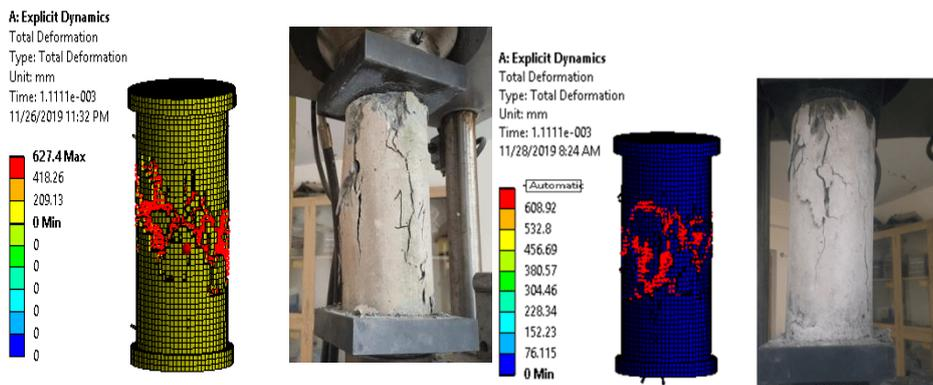
**Figure 3.** Comparative analysis of concrete cylinder (FRC 2 & FRC 3)
