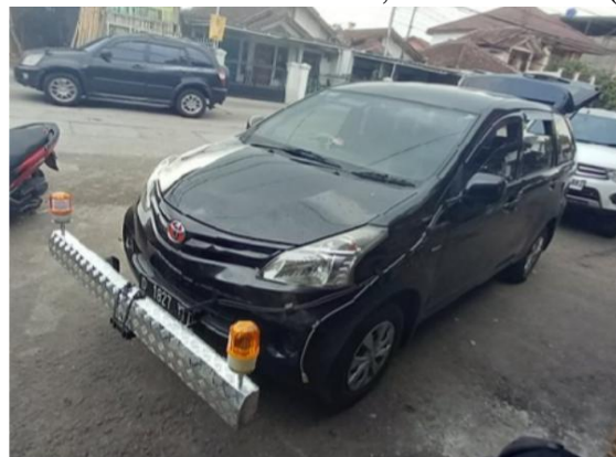
Figure 5. The Ultrasonic Surface Rough meter that has been installed on the vehicle
