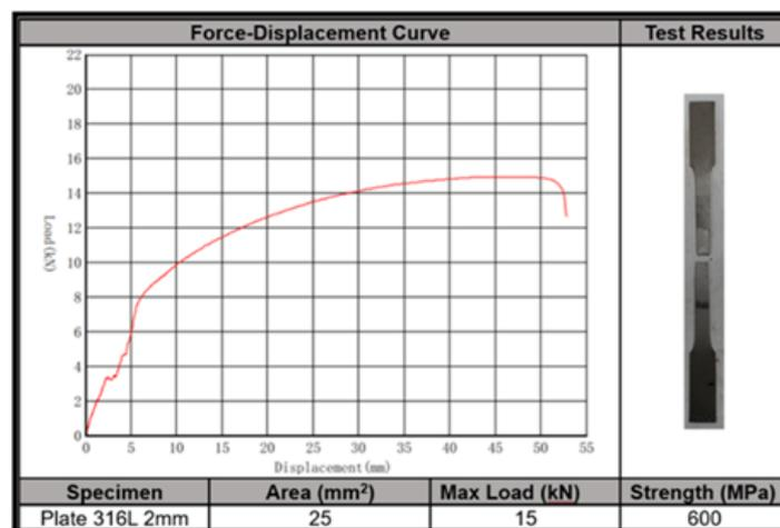
**Figure 5.** Force-displacement curve
