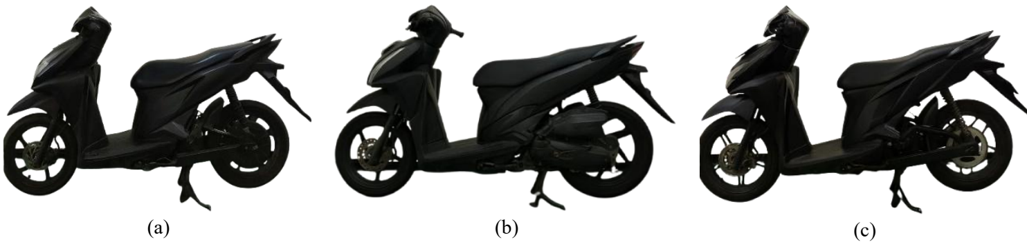
Figure 5. Electric two-wheeler conversion results: (a) hub / in-wheel (b) CVT (c) gear ratio
