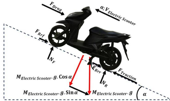
Figure 2. Dynamic Longitudinal Free Body Diagram
