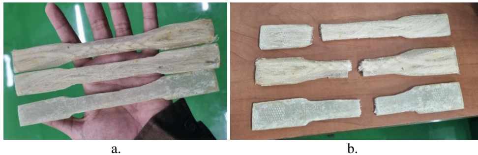
Figure 4. a. Dog-bone specimens for tensile testing; bottom to top: fiberglass–resin, unbraided pineapple–resin, braided pineapple–resin; b. Post-tensile test specimens showing failure patterns; bottom to top: fiberglass–resin, braided pineapple–resin, unbraided pineapple–resin
