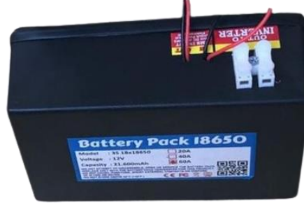
Figure 2. Li-ion battery pack used in the system
