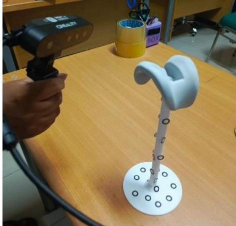
Figure 6. Total Knee Replacement (TKR) implant scanning process using AESUB spray [23][24].
