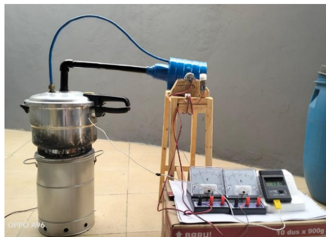
Figure 3. RDF-based Power Generation Machine Prototype
