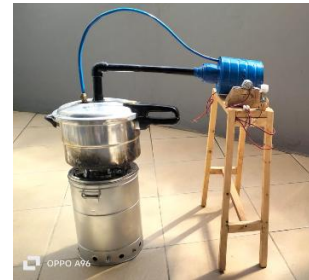
Assembling it into an RDF-based power generating machine
