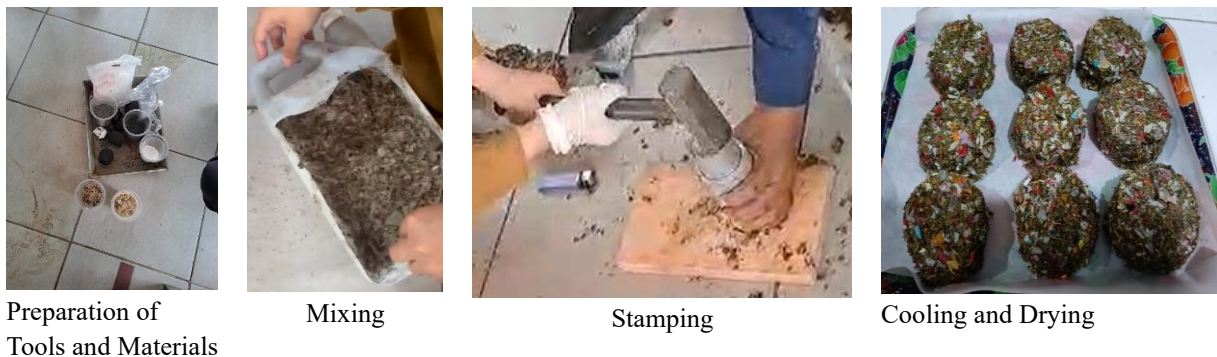
Figure 1. RDF Briquette Making Process
