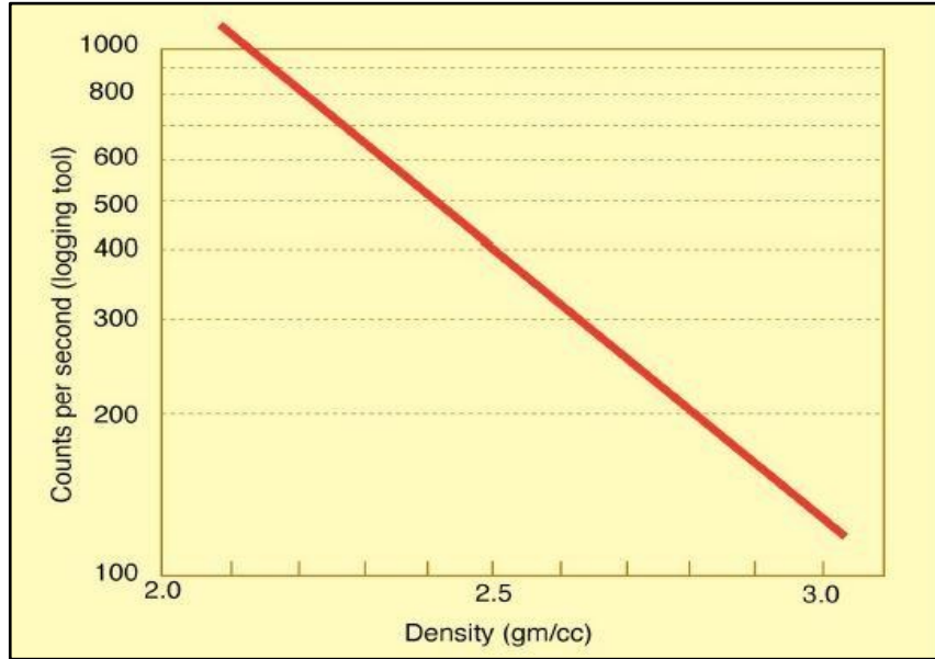
Figure 3. Relationship between CPS units and gr/cc
