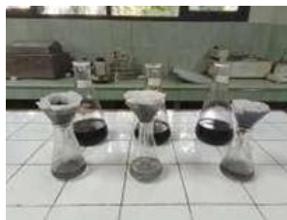
Figure 4. MnO 2 –Carbon composites obtained from hydrothermal synthesis (Source: Authors’ documentation)
