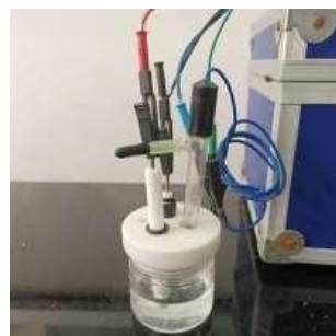
Figure 6. Three-electrode system for electrochemical testing (Source: Authors’ documentation)
