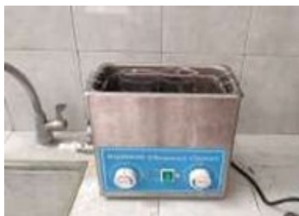
Figure 1. Washing process of carbon using ultrasonic cleaner (Source: Authors' documentation)
