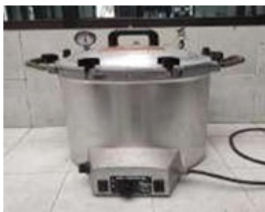
Figure 3. Hydrothermal synthesis of MnO 2 –Carbon using autoclave (Source: Authors’ documentation)
