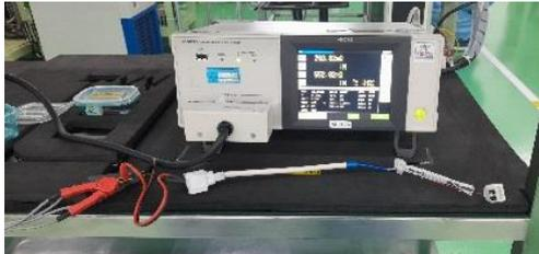
Gambar 2 Pengecekan *LCR meter quality*
