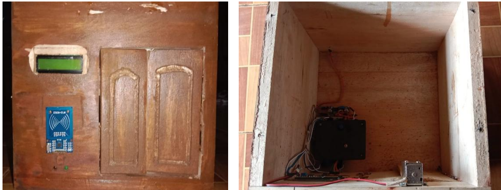
Figure 4. Smart door lock props on magnetic field material based on RC522 RFID sensor and Arduino Uno.
